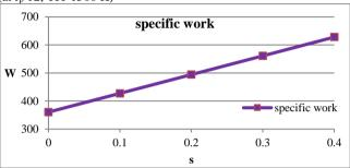
Fig 9 Effect of specific steam rate per kg of air on specific work output (at r<sub>p</sub> 12; TIT 1500 K)
