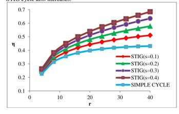
Fig 2: Effect of pressure on cycle efficiency (at TIT 1500K)
