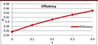
Fig 8 Effect of specific steam rate per kg of air on cycle efficiency (at r<sub>p</sub> 12; TIT 1500 K)
