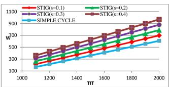
Fig 6 Effect of TIT on specific work output (at r<sub>p</sub> 12)
