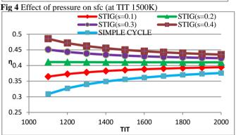
Fig 5 Effect of TIT on cycle efficiency (at rp 12)
