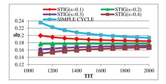
Fig 7 Effect of TIT on sfc (at rp 12)
